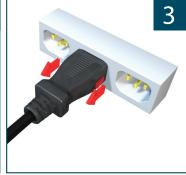
To release, pull on the red tabs and remove cord.
