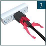
Tighten red nut while pushing towards PDU to maintain insertion. After initial resistance is felt, tighten only another  $^{1}\!\!/_{4}$  to  $^{1}\!\!/_{2}$  turn. Do not over-tighten.
