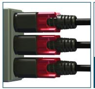
Align nuts as shown to maximize clearance in ganged receptacles.
